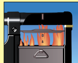
STAGE 3 - In under a minute, the fire extinguishing plate drops on to the liners.
